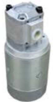
1.6-2.5 kW (12-24 V) Pompa: GR 10, X001G 0.8 cc/dev-10 cc/dev
